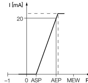
Fig. 10: Behavior of the current output (0...20 mA)
