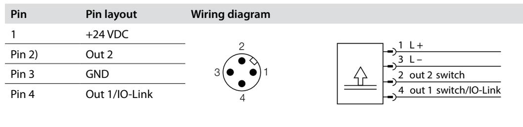
Fig. 13: Wiring diagram PS...D...2UPN...
