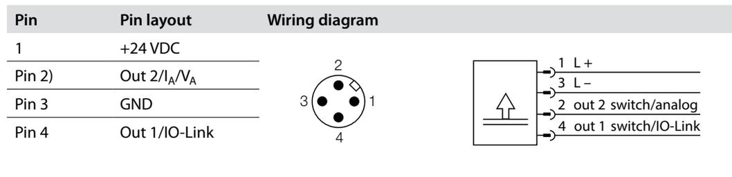
Fig. 14: Wiring diagram PS...D...LIUPN...
