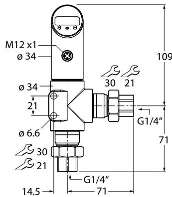
Fig. 1: Dimensions – PS...D-501L...
