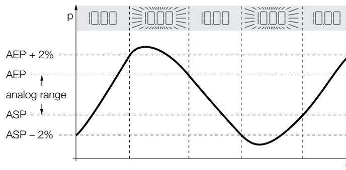
Fig. 15: Display – Value within the set measuring range
