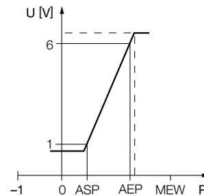
Fig. 12: Behavior of the voltage output (1...6 V)
