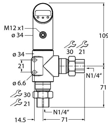
Fig. 2: Dimensions – PS...D-502L...
