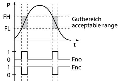
Fig. 7: Behavior of the switching output (window function)
