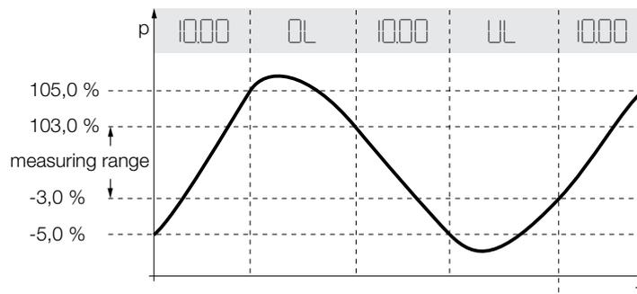
Fig. 16: Display – Value outside the set measuring range
