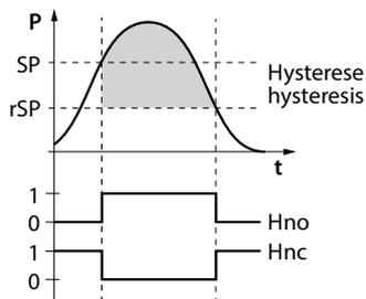
Fig. 8: Behavior of the switching output – Hysteresis function
