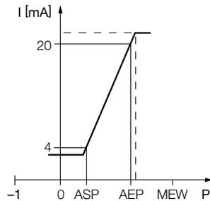
Fig. 9: Behavior of the current output (4... 20 mA)
