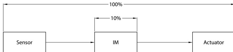
This means that the failure limit value must be less than or equal 100 FIT. ( $\text{PFH} \leq 10^{-7} \text{ h}^{-1}$ )
