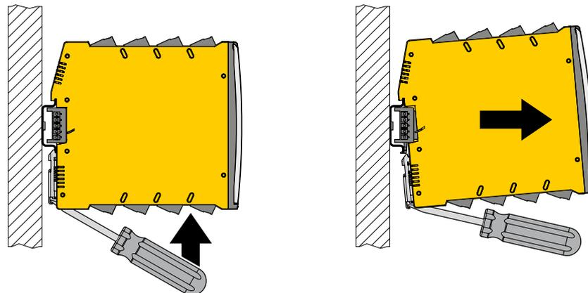
Fig. 4: Remove device
