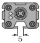
A guide slot at the sensor backside takes the sliding blocks.
