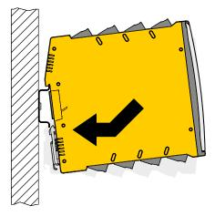
Fig. 1: Fasten the device
