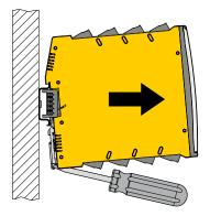
Fig. 4: Remove device
