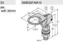
Mounting bracket, stainless steel, for M10 x 1.5 thread, thread length 30 mm
