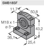
3052519 Mounting bracket, PBT black, for sensors with 18 mm thread, rotatable
