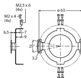
Stainless steel flex mount coupling for hollow shaft encoders, reference diameter 63 mm, for applications with high demands on accuracy
