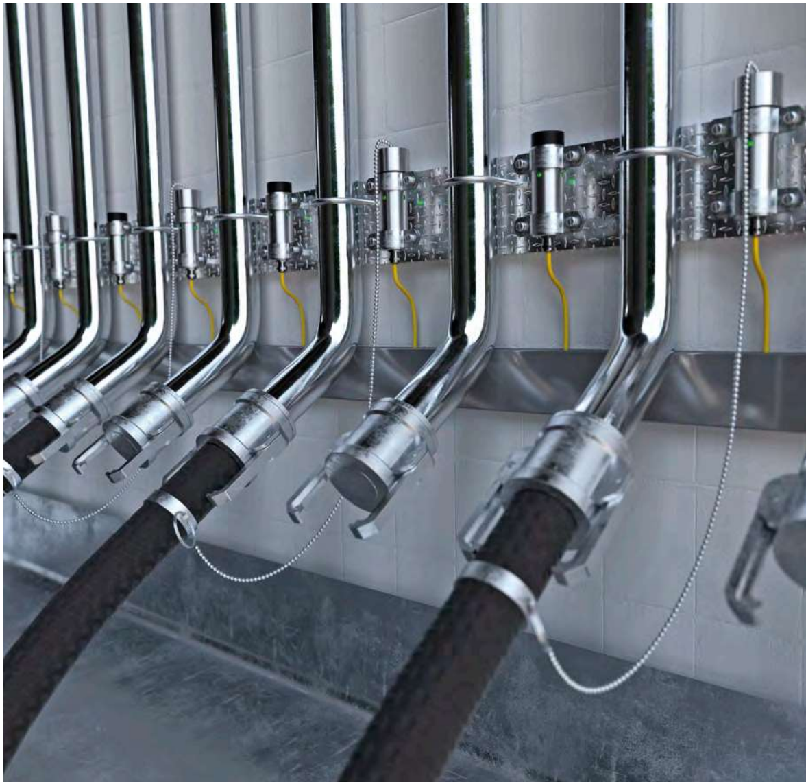
RFID is a simple and reliable solution for the identification and verification of modules, containers or hoses, as shown here
